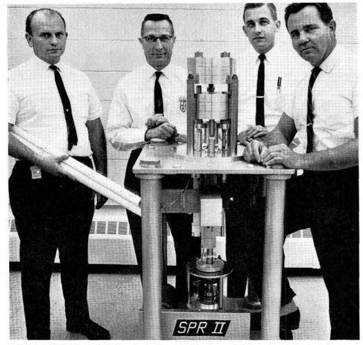
SPR-II MOCK UP, built full scale in Sandia's Development Shops, has helped designers visualize design, control, and operational features. From left are Dick Coates, project engineer; Willard Schmidt, nuclear designer; Jon Reuscher and Don Cox, mechanical designers. All are in Reactor Development Division 5223.
